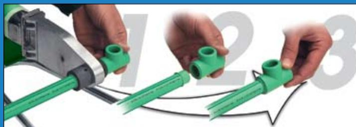
**Figure 2** Socket fusion procedure
